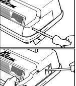
Remove the door by removing the hold down screw located on side of power head.
